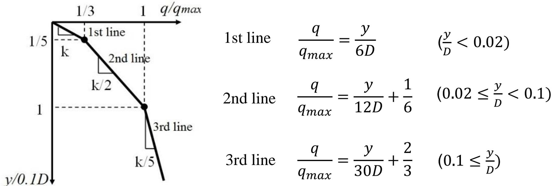
Fig. 11 Pile end resistance (R-y curve)
