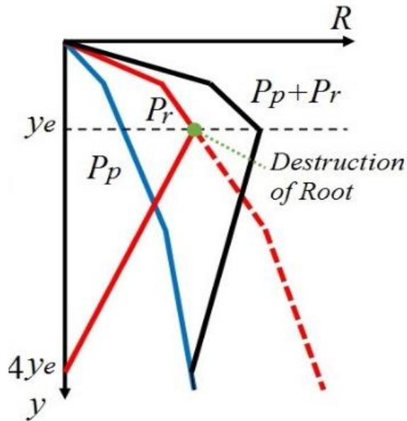
Fig. 11 Pile end resistance (R-y curve)
