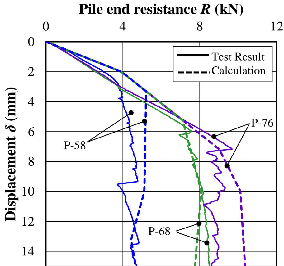
Fig. 13 Comparison between test and calculation results (**P-series**)
