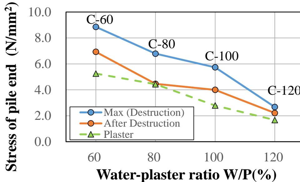
**Fig. 7 Relationship between water-plaster ratio and destruction stress of pile end (C-series)**
