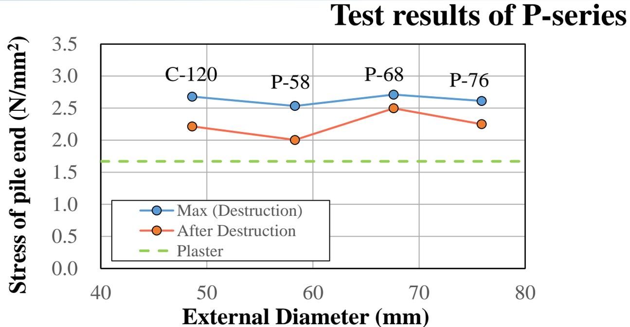
**Fig. 8 Relationship between external diameter of the end plate and destruction stress of pile end (P-series)**
