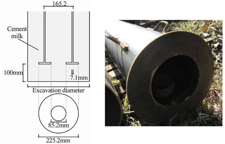
Fig. 9 Pile tip shape of field test
