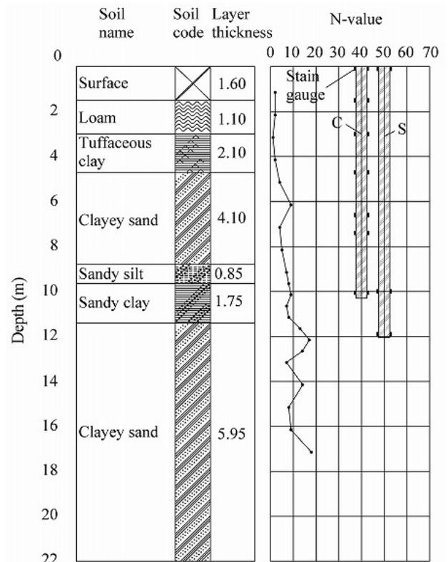
Fig. 10 Boring logs of field test
