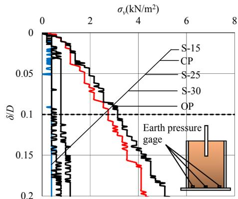
Fig. 6 Relationship between displacement and vertical earth pressure (S-series)
