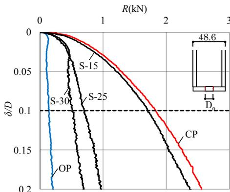
Fig. 4 Relationship between displacement and pile end resistance (S-series)
