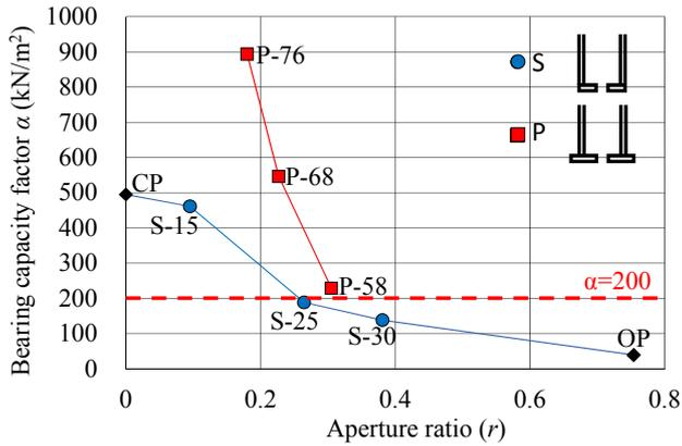
Fig. 8 Relationship between a bearing capacity factor  $\alpha$  and aperture ratio  $r$
