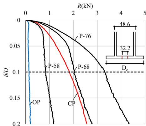
Fig. 5 Relationship between displacement and pile end resistance (P-series)
