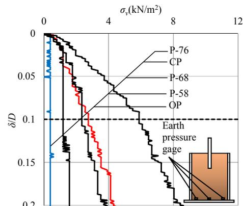
Fig. 7 Relationship between displacement and vertical earth pressure (P-series)
