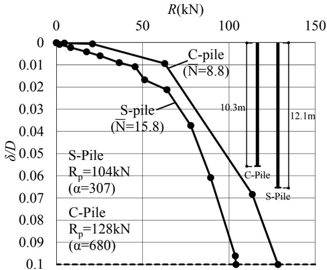
Fig. 11 Relationship between displacement and pile end resistance (S-pile and C-pile)
